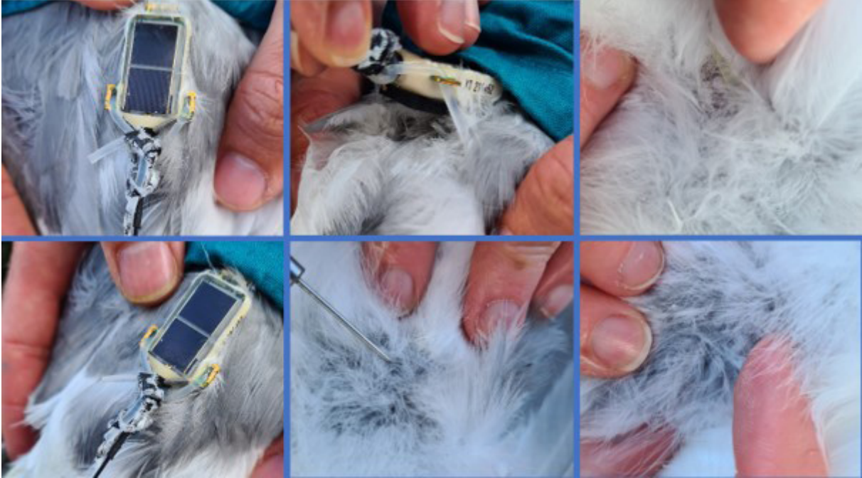
Figure A5. Photographs of the device and harness of Kittiwake 214452 showing that the back knot was still intact but the Tesa tape that had been put on around the silicone cord knot on the 25/06/2023 had been pecked at. There were no signs of abrasions from the silicone cord harness.
